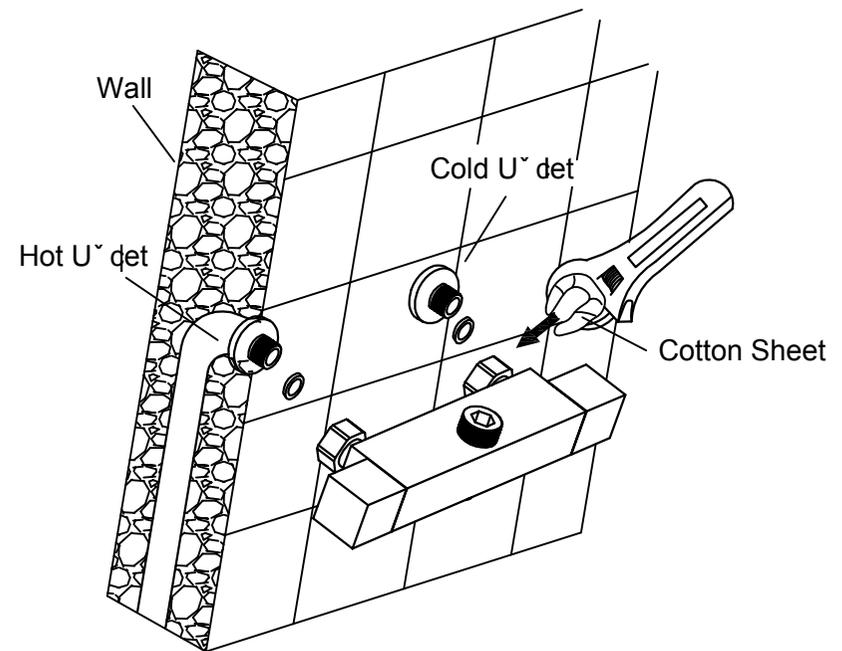
3. Measure the installation height of the shower kit. Mark two holes in the required position. Drill holes properly with electric drill and place the wall plugs into the holes. Fit the cap into the fixing plate.
