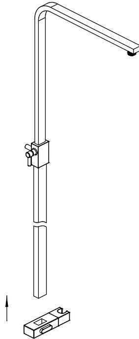
**Step 2:** Put the adjustable holder onto the rail slider.
