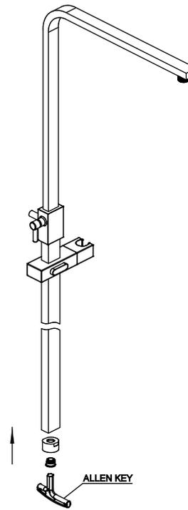
**Step 3:** Screw on the connector back to the rail slider.
