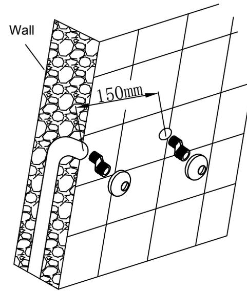
2. Fix the shower valve to the off-set connector using an adjustable spanner. Please use a cotton sheet inside of the spanner to avoid any scratches. Make sure hot water outlet is on the left and cold water outlet is on the right, otherwise it will affect the performance.
