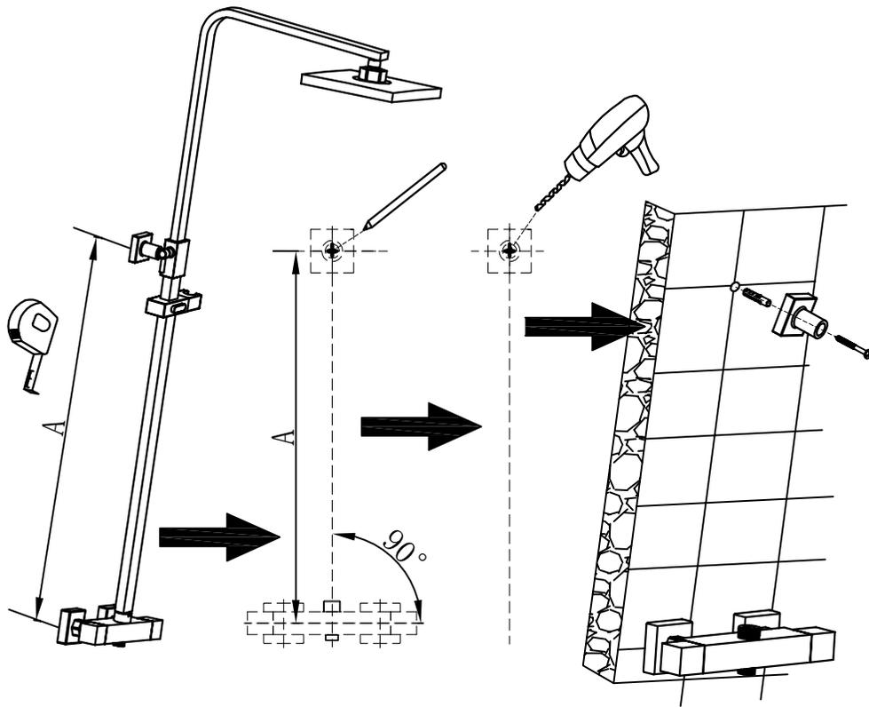
4. Align the shower valve and connector and tighten the nuts using an adjustable spanner. Fit screw to the fixing plate with allen key then secure the rail to the wall. Finally connect the hand shower to the flexible hose, flexible hose to the mixed water outlet and shower head to the top of sliding rail.
