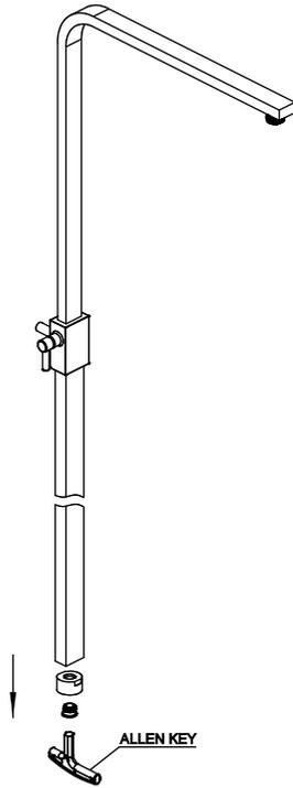
**Step 1:** Screw off the connector using Allen key.
