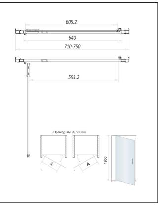
Dimensions (measurements in mm)
