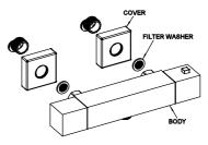
Step 3: Attach the covers against wall, place filters into the inlets. Then fix mixer onto the wall with spanner, checking for leakage.
