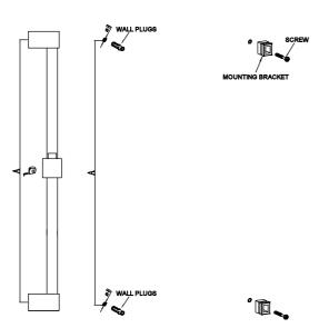
Step 4: Measure the center distance of the sliding rail with a tape measure, Drill two holes of Ø8mm with depth of 40mm,tap in wall plugs.
